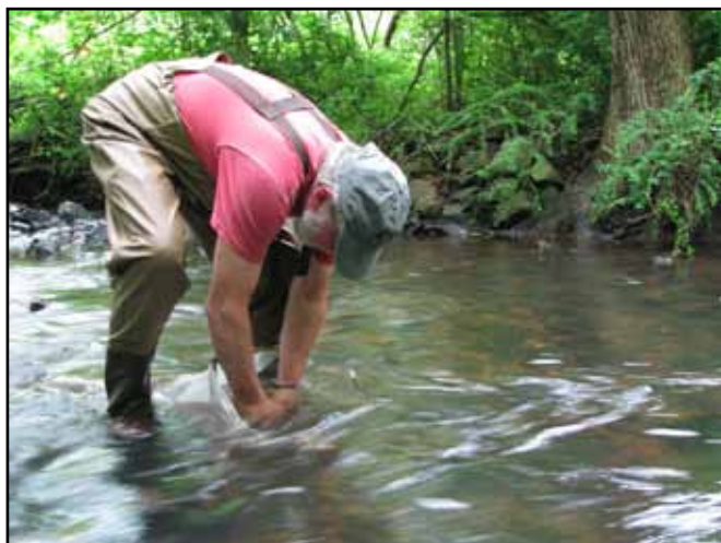
Dr. Pollock rubs the rocks just upstream of his sampling net to detach any MIVs. The streamflow will carry them into his net.
