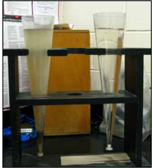
A comparison photo of sewer water coming into the Woodland Plant (left), and treated water leaving the plant (right). Photo by L. Kelm.
