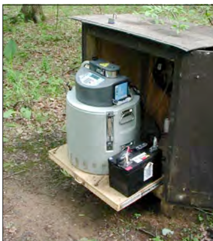
An ISCO automated sampling unit, one of which is located at each of the five streams which flow into Great Swamp.
